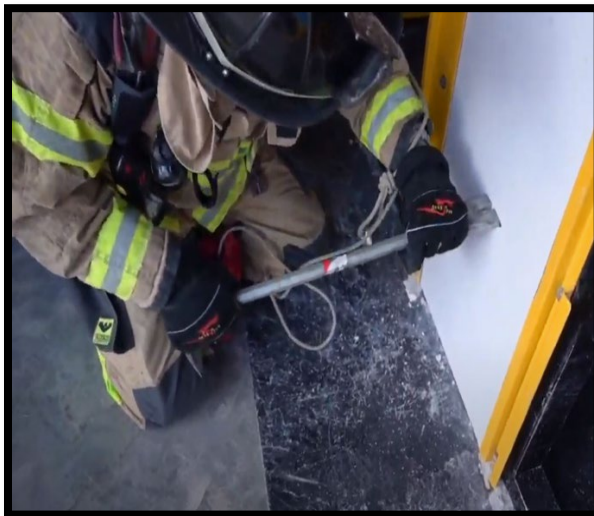
(FIGURE 3, 4) AN ANCHOR AROUND A STUD CAN BE A VERY SECURE ANCHOR, BUT IN THE ABSENCE OF STUDS, A CARABINER ON THE DRYWALL WILL WORK.
